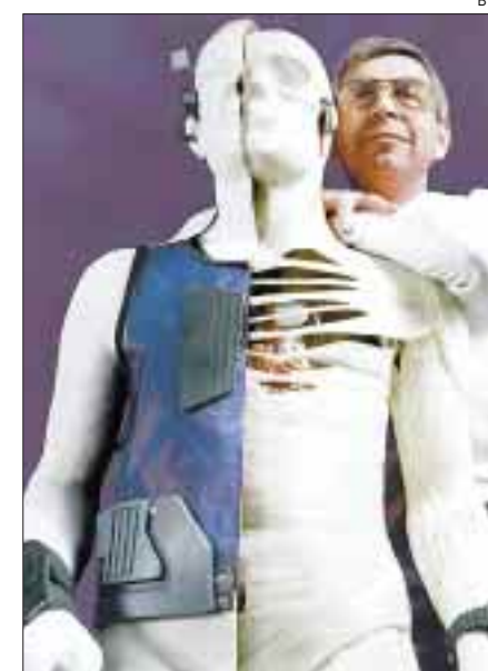
WIRED MAN: scientists at BT have developed a body-worn computer with 'distributed body furniture' such as a watch-phone and arm computer
