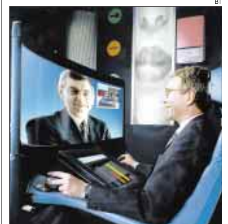
SMART SPACE: the office workstation of the future, as designed by BT. Wrap-around screen for video-conferencing and touch-sensitive computer keyboard
