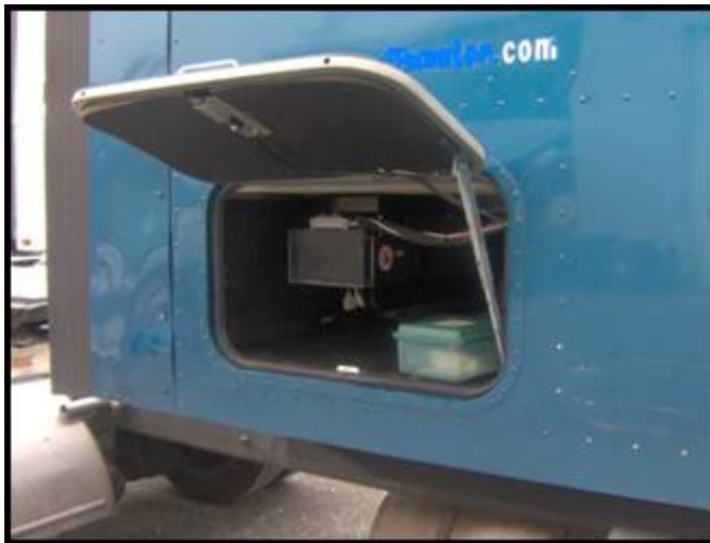
Figure 5. Photo. Encased computer and external hard drive installed in the truck's rear storage compartment.
