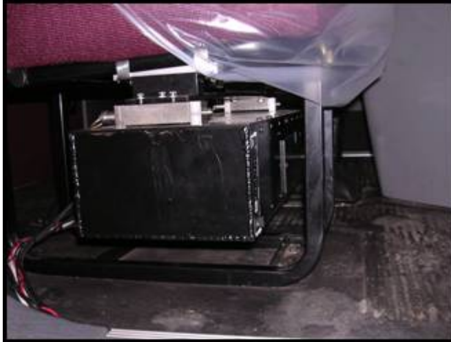
Figure 4. Photo. Encased computer and external hard drive installed under the passenger seat.
