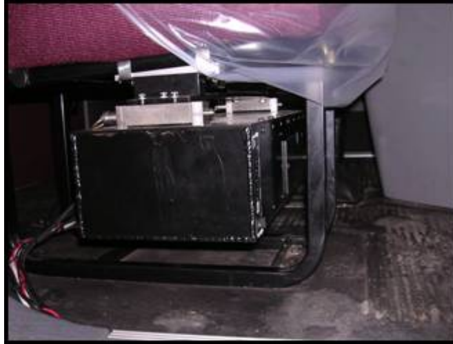
Figure 1. Photo. Encased computer and external hard drive installed under the passenger seat.
