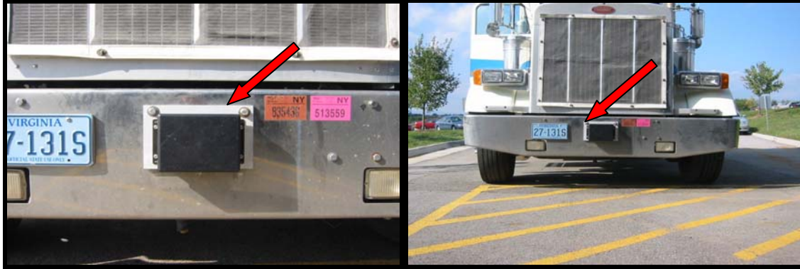
Figure 7. Photo. VORAD unit on the front of the truck.
