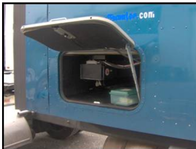
Figure 2. Photo. Encased computer and external hard drive installed in the truck's rear storage compartment.
