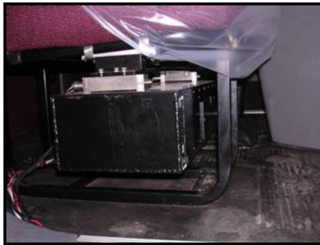
Figure 1. Photo. Encased computer and external hard drive installed under the passenger seat.
