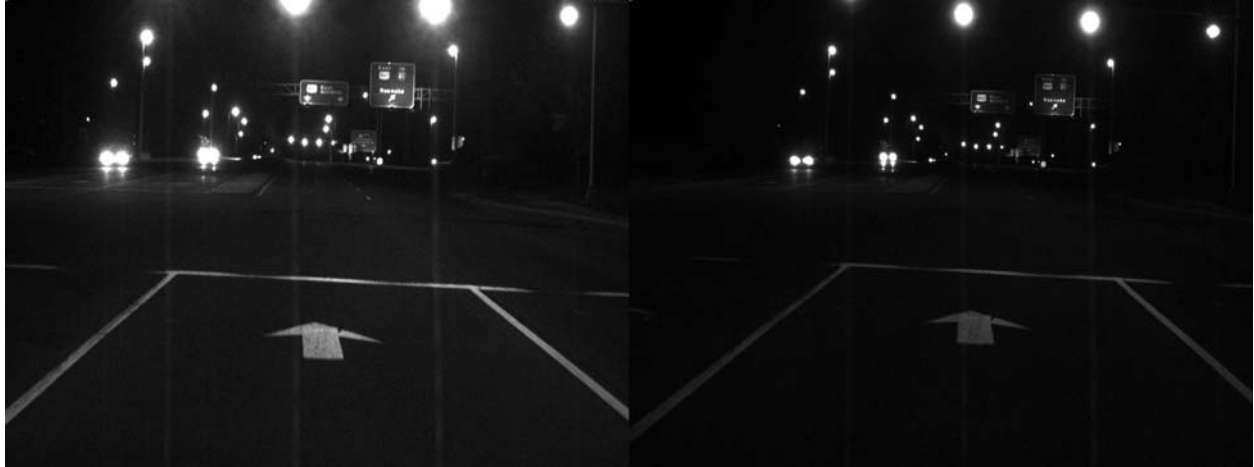
Figure 11. Photo. Comparison between higher gain/shutter (left) and lower gain/shutter (right).
