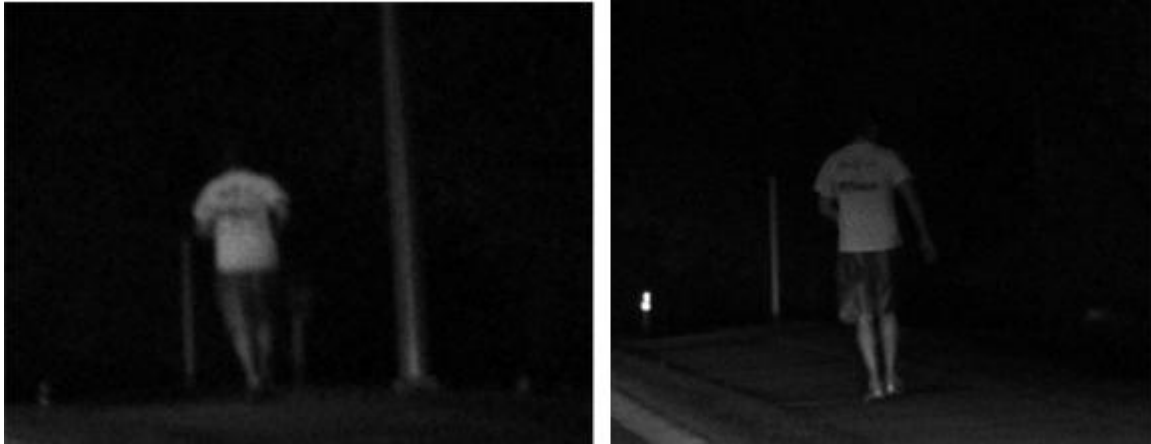
Figure 1. Photo. Luminance changes in pedestrian from overhead lighting (left) to no overhead lighting (right).
