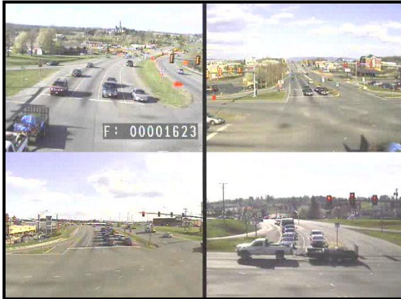
Figure 10. Photo. Video quadrants from camera units mounted on intersection mast-arms.
