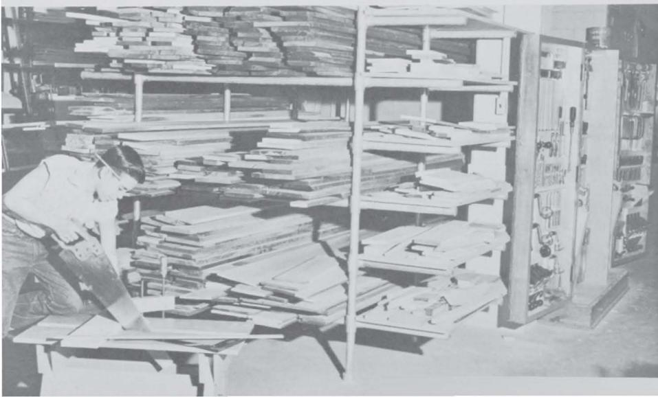
**A Saw Horse** (Figure 71) with a flat top is helpful in the wood area. The saw horse should be built sturdily with a top approximately 12" wide, 30" long, and 18" high, with a 2" slit through the center of the top board. By providing students with a saw horse, they can be taught the proper way to hold and use the cross-cut and rip saws.
