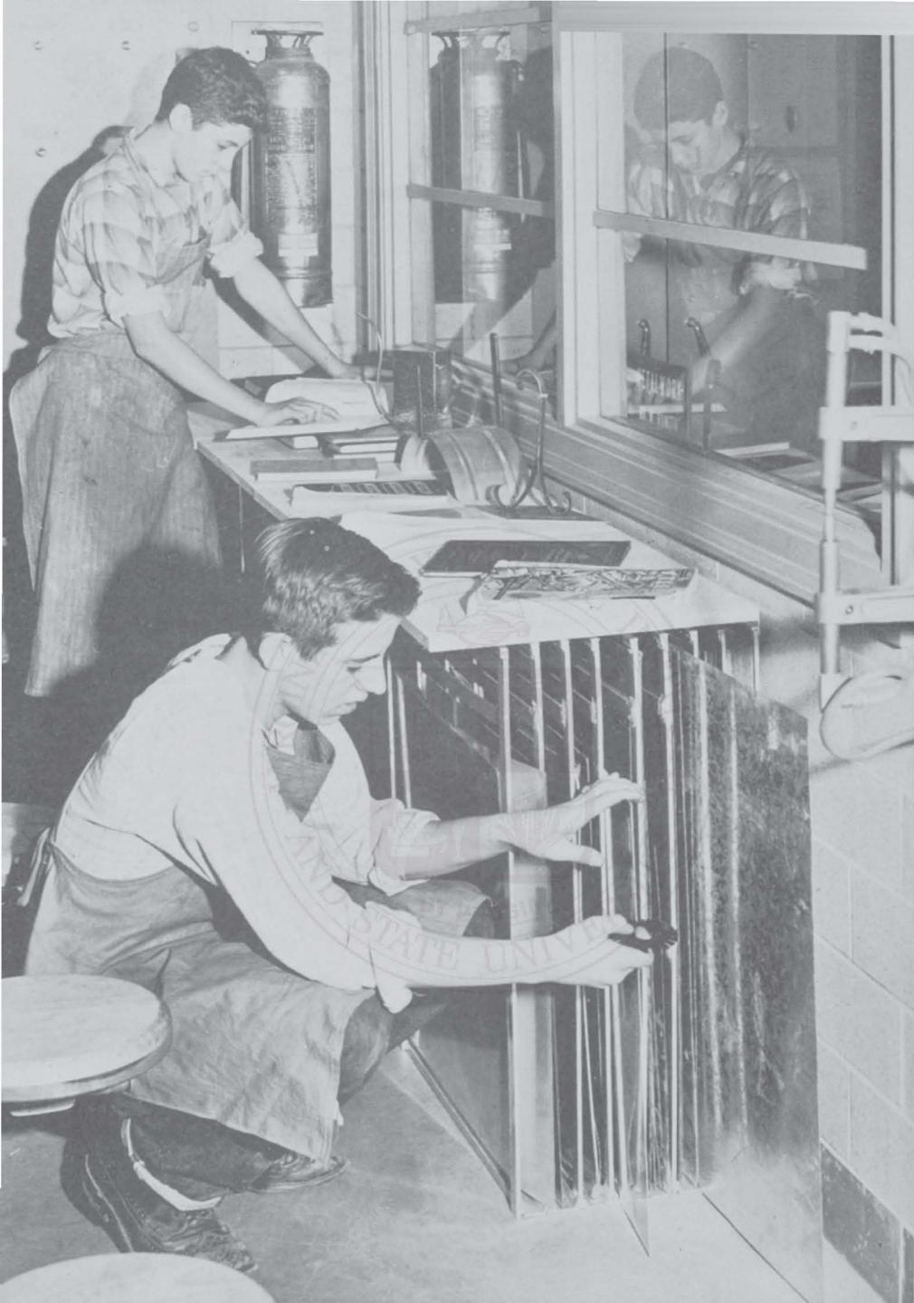
Figure 73. Vertical Sheet Metal Storage Rack
