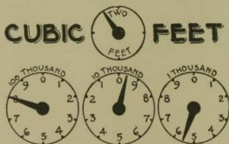
FIG. 42.—Gas meter index reading 79,500 cubic feet.
