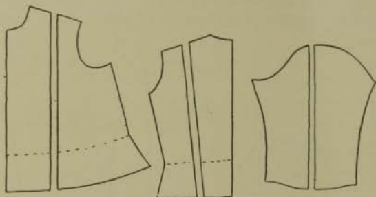
FIG. 65.—Method of cutting and opening a shirt-waist pattern to throw in fullness. This method of putting more fullness into a shirt-waist pattern also increases the length of the shoulder. The line of opening should extend through about the center of the shoulder. It is often necessary to increase the size of the arm-hole to make it correspondingly larger. The sleeve may be opened along the center.
