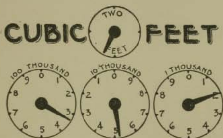
FIG. 41.—The index of a gas meter. Each dial is marked with the volume of gas passed a revolution. The smaller top dial, which is marked "Two Feet" inside of the circle, is generally called the "testing circle" or "proving head" and is used principally in testing the meter.
