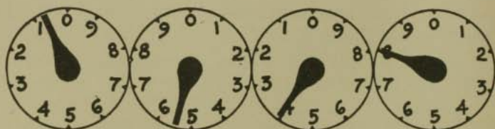
FIG. 44.—Dial of a watt-hour meter. In this dial the hand on the second circle from the right is slightly in advance of its proper position on its shaft. The reading is the same as in Fig. 43, namely, 538 kilowatt hours, although at a glance it might be incorrectly read as 548 kilowatt hours.
