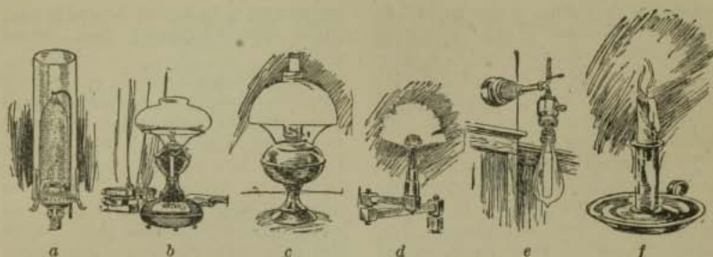
a. Incandescent gas or gasoline gas at $1 per 1,000 ft. costs \frac{1}{2} c. per hour. Equals breath of 3 persons; b. Acetylene gas costs \frac{1}{2} c. per hour. Equals 2 or 3 persons; c. Kerosene lamp costs \frac{1}{2} c. Equals 7 or 8 persons; d. Open flame gas costs \frac{1}{2} c. Equals 6 persons; e. Electric bulb costs 1\frac{1}{2} c. Consumes no oxygen; f. Candles cost 6\frac{1}{2} c. Each candle equals 12 persons.
