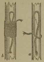
Is used for fastening broken sticks or rods after serving them with several turns of the cord which should never overlap. Before beginning the serving make a loop a little longer than the proposed extent of the turns (a Fig. 3). When the serving is finished pass the end of the cord through this loop, and by pulling in its free end the other is drawn within the serving and made secure (b Fig. 3).
