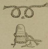
in the left hand, turn the free end under it, and put it over the thumb; repeat this, and the hitch is made. (Fig. 5.) When the clove-hitch is made on the standing part of the rope, after it has passed around a post or box, it is called two half-hitches, and is the best method of fastening boxes or bundles. In this case it should never be fastened to the cord at right angles to its own, but that in a line with it. (Fig. 6.)
