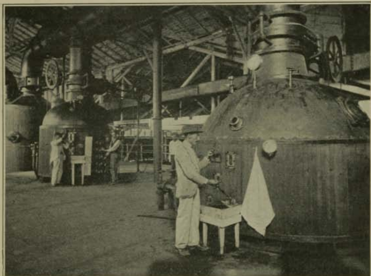
FIG. 33.— Vacuum pans in sugar factory. Operator in foreground using "proof stick" to withdraw test portion of contents (American Photo Co., Havana).
