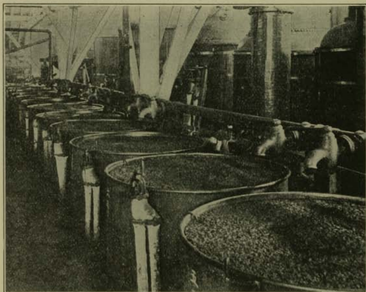
FIG. 37. — Clarifying cane juice (American Photo Co., Havana).
