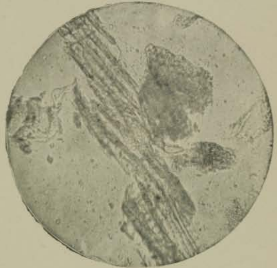
FIG. 266.—Pine Sawdust, \times 110 . Finely ground.
