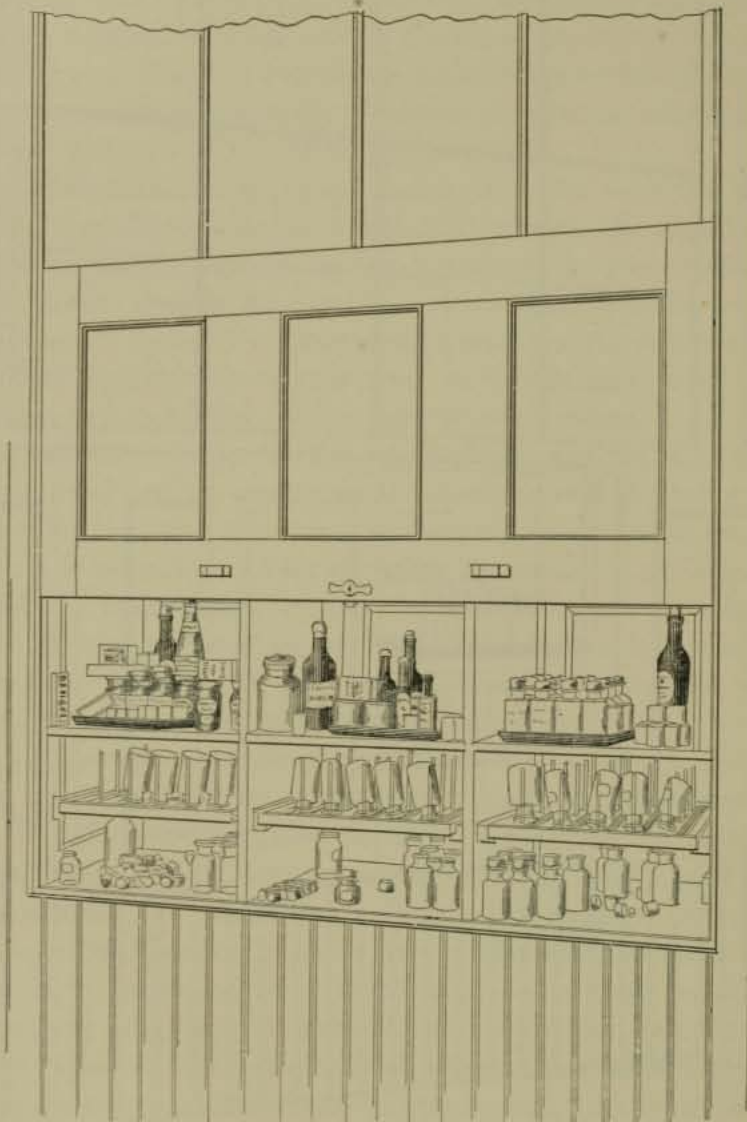
FIG. 2.—Inspectors' Lockers. Front View. The lockers are accessible to the analyst in the laboratory by a single sliding-sash front, provided with a spring lock. The removable sliding-racks are convenient for returning clean sample bottles.
