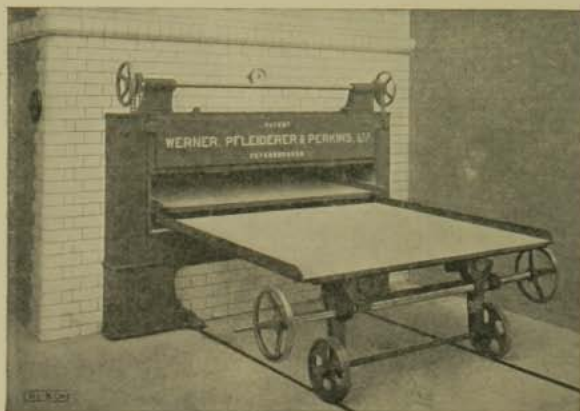
FIG. 81. OVEN WITH SPLIT DRAWPLATE.
