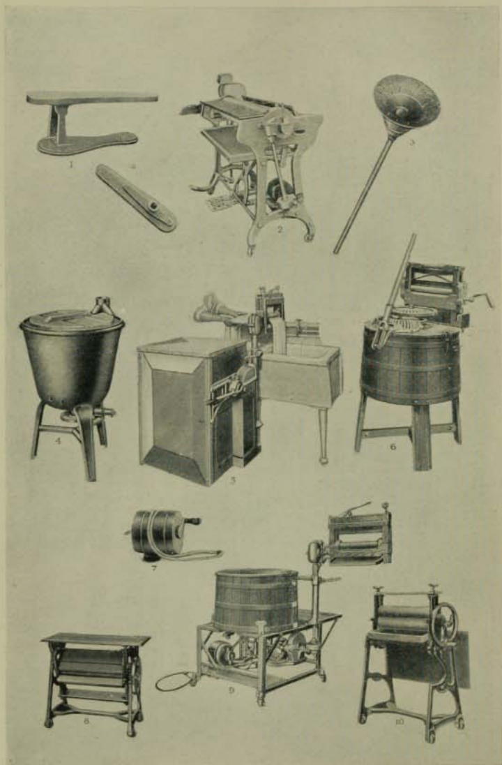
1. Ironing Sleeve. 2. Electric Ironing Machine. 3. Vacuum Clothes Washer. 4. Gas-heated Copper. 5. Electric Washing Machine, showing Wringer in operation. 6. Hand Washing Machine. 7. Clothes-line Protector. 8. Table Mangle, as Table. 9. Electric Washer and Wringer. 10. Electric Washer and Wringer.
