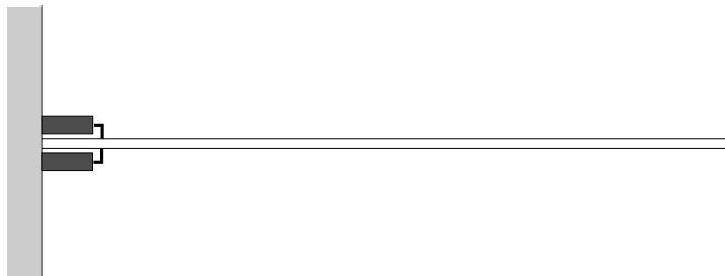
Figure 8. Cantilever beam with magnetostrictive actuators.
