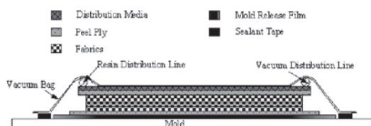
Figure 7. Schematic of the VARTM Process
