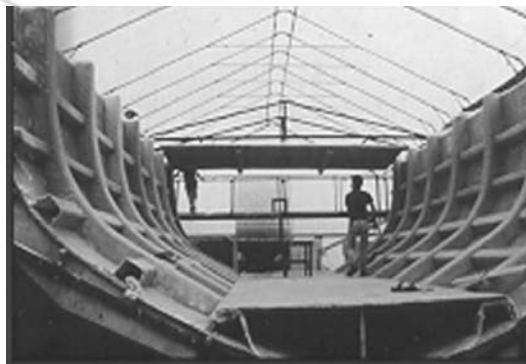
Figure 6. Huge Boat Hull Manufactured Using VARTM (Advanced Projects Group, 2009)
