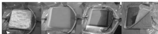
Figure 8. VARTM Process at Small Scale - from Material Arrangement to Resin Infusion and Demolding
