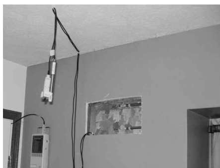
Figure 5. Data Logger and Interior Climate Sensors, Kearney
