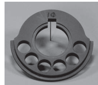
Figure 4: Typical Rotary Displacer Segment
