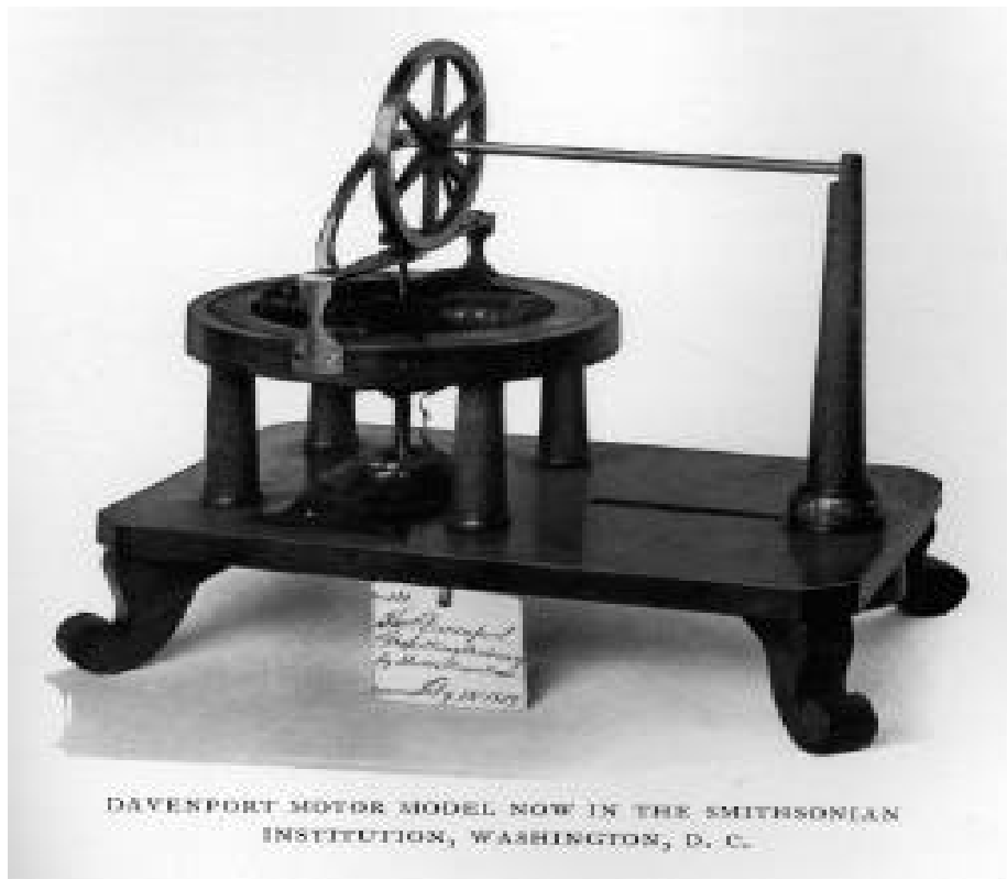
Figure 1. A model of Davenport's motor, that was patented in 1837. (Davenport 1929 p. 144)
