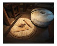
In examining a set of millstones, one will see that the bottom surface of the runner stone and the top surface of the bed stone are grooved or "furrowed," in a pattern which causes the meal to flow away from the center of the stones to their outer edge. The layout of the furrows is referred to as the "dress" which is generally one of two patterns: (a) *the sickle dress* or (b) *the quarter dress*. Both stones in the McCormick Mill have a quarter dress. See next page.
